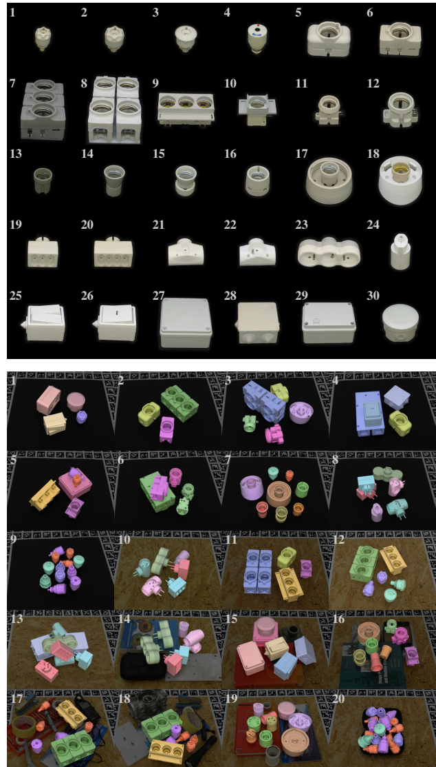
Figure 2. T-LESS includes training images and 3D models of 30 objects (top) and test images of 20 scenes (bottom) – shown overlaid with colored 3D object models at the ground truth poses. The images were captured from a systematically sampled view sphere around an object/scene and are annotated with accurate ground truth 6D poses of all modeled objects.
