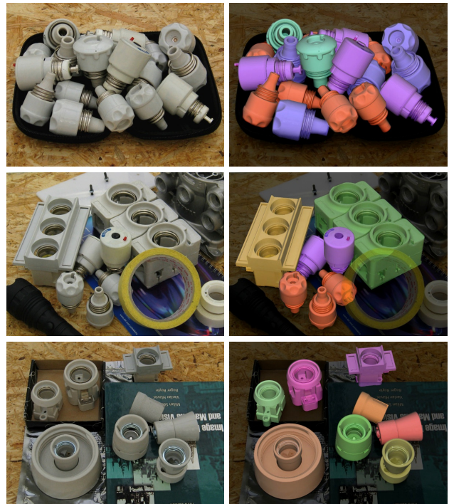
Figure 1. Examples of T-LESS test images (left) overlaid with colored 3D object models at the ground truth 6D poses (right). Instances of the same object have the same color. The goal is to find instances of the modeled objects and estimate their 6D poses.
