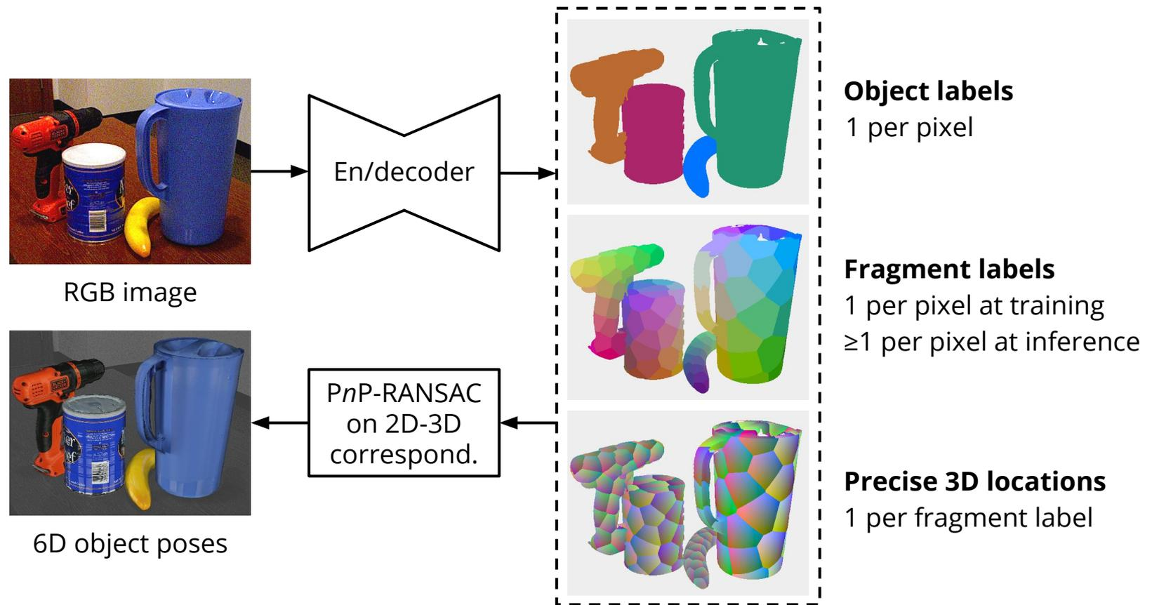
**Potential 2D-3D correspondences** are established by linking each pixel with the predicted 3D locations on possibly multiple fragments.
