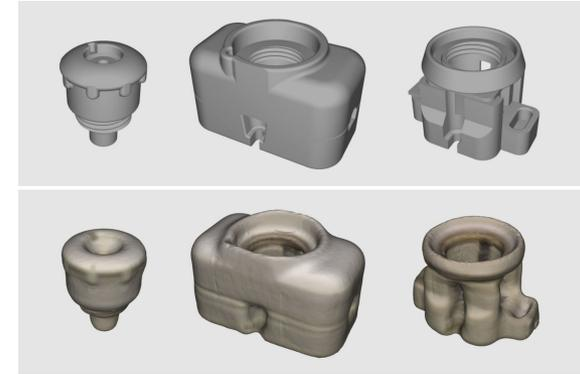
CAD and reconstructed 3D object models
